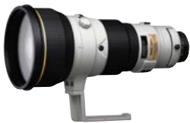
Some long lenses have with a lens collar with a tripod mounting foot. To switch one of these lenses from horizontal to vertical, you loosen a screen on the collar and rotate the camera. This keeps the center of gravity of these heavy lenses over the tripod. Courtesy of Canon.
