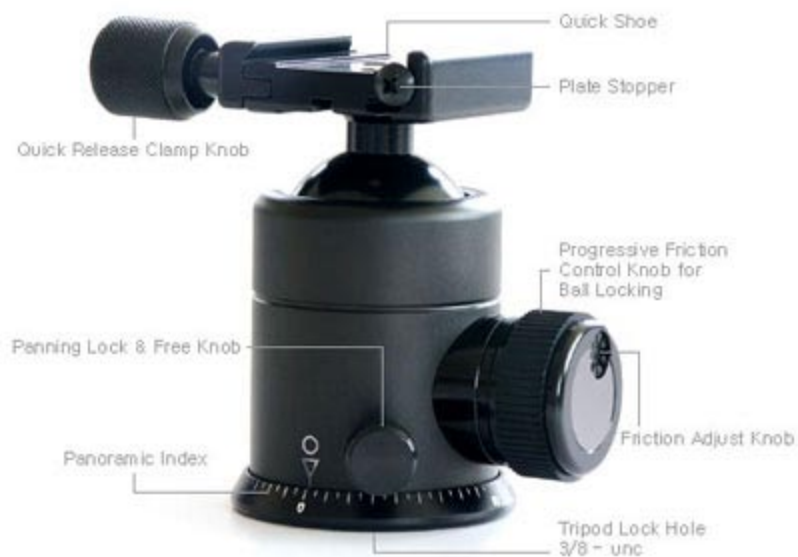
The parts of a Markins ball head. Courtesy of Markins.
