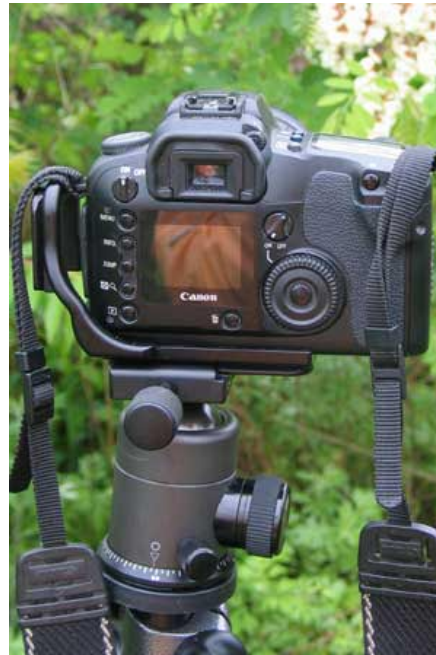
Using an "L" plate, a camera mounted using the horizontal plate (left) or the vertical plate (right).
