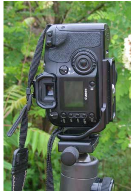
Using an "L" plate, a camera mounted using the horizontal plate (left) or the vertical plate (right).
